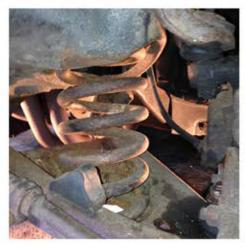
Once your vehicle is safe and secure, begin by removing the factory coil springs. To avoid possible clearance issues, your factory bump stop may need to be removed.
